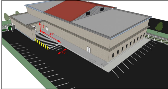
Figure 5.1.12.B.2: Loading Area Configuration
